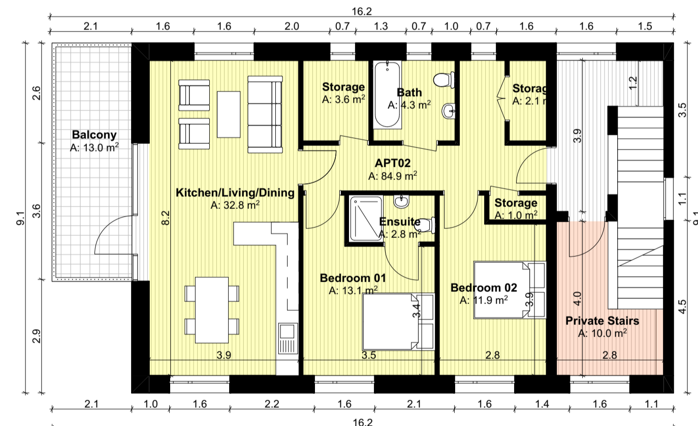
Second Floor Plan SCALE 1:100 GFA: 84.9 m²
